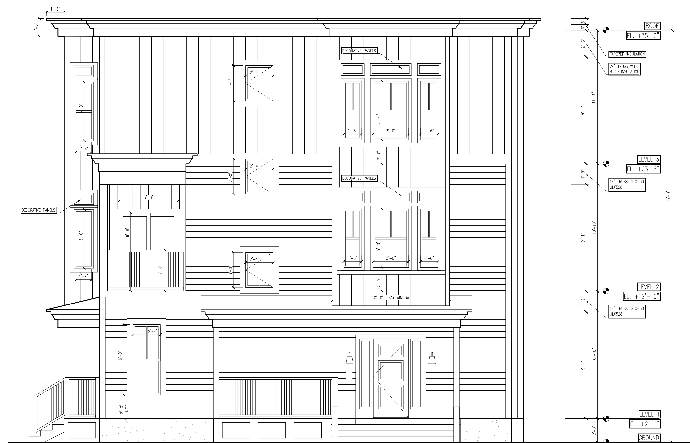
2 PROPOSED ALVARADO AVE. ELEVATION SCALE: 1/4" = 1'-0"
